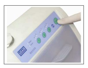
8. Press the air button if you wish to run a cycle of only air through your handpieces. This process removes any excess lubrication fluid from the turbine
